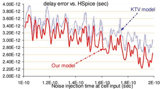
Figure 4. Absolute errors in calculated delay for a min size inverter
